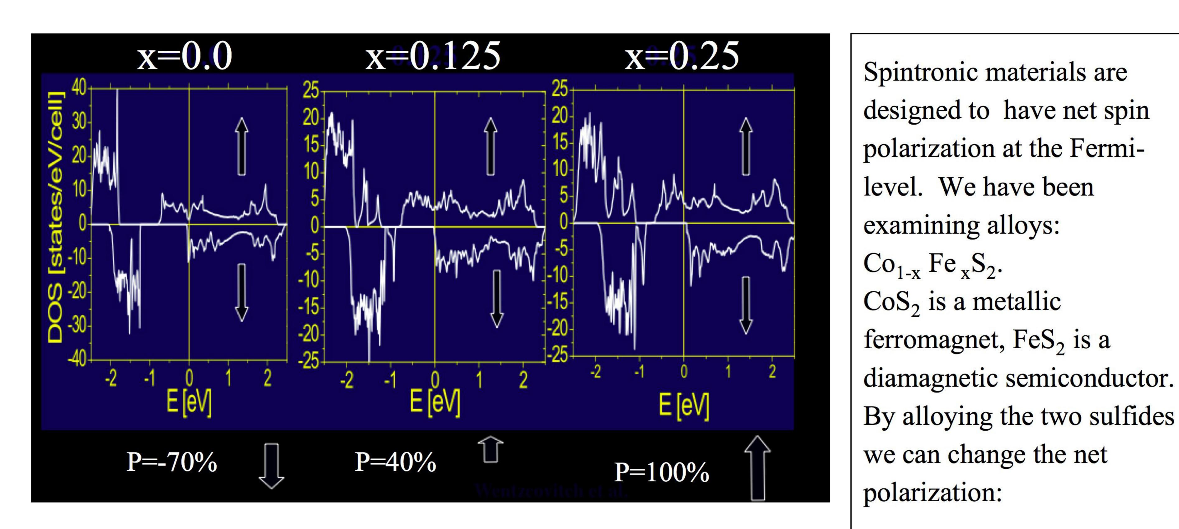
Density of states for  $Co_{1-x}$  Fe  $_xS_2$ . The energy zero is the Fermi-level. For x=0, the material is a ferromagnetic metal with "negative" spin polarization, i.e., the polarization at the Fermi-level is opposite to the majority spin. The change in sign of the polarization as a function of x has been observed experimentally. It was predicted before the experiment.
