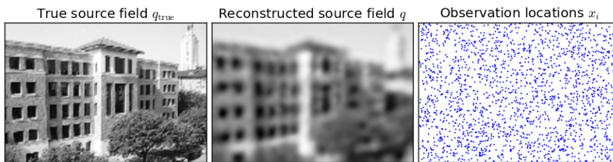
FIG. 1. Left: True source field q_{\text{true}} used for all inversions. Center: Reconstruction q for the case of n_{\text{obs}} = 2000 observations with regularization parameter \alpha = 10^{-8} and mesh size h = \sqrt{2} \cdot 10^{-2} . Right: Observation locations x_k , denoted by dots.
