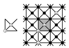
Fig. 2. Lattice notation. To the left, an irreducible unit cell is depicted. Each node is marked with its type,  $\kappa$ . To the right, the cell m = [0,0] is marked in grey. The node marked "a" is a node of type  $\kappa = 1$  in cell m = [0,0]. Thus node "a" is labeled (1,[0,0]). Node "b" is of type  $\kappa = 2$  and has the label (2,[0,0]). Node "c" is labeled (1,[0,-1]), and node "d" is labeled (2,[1,1]).
